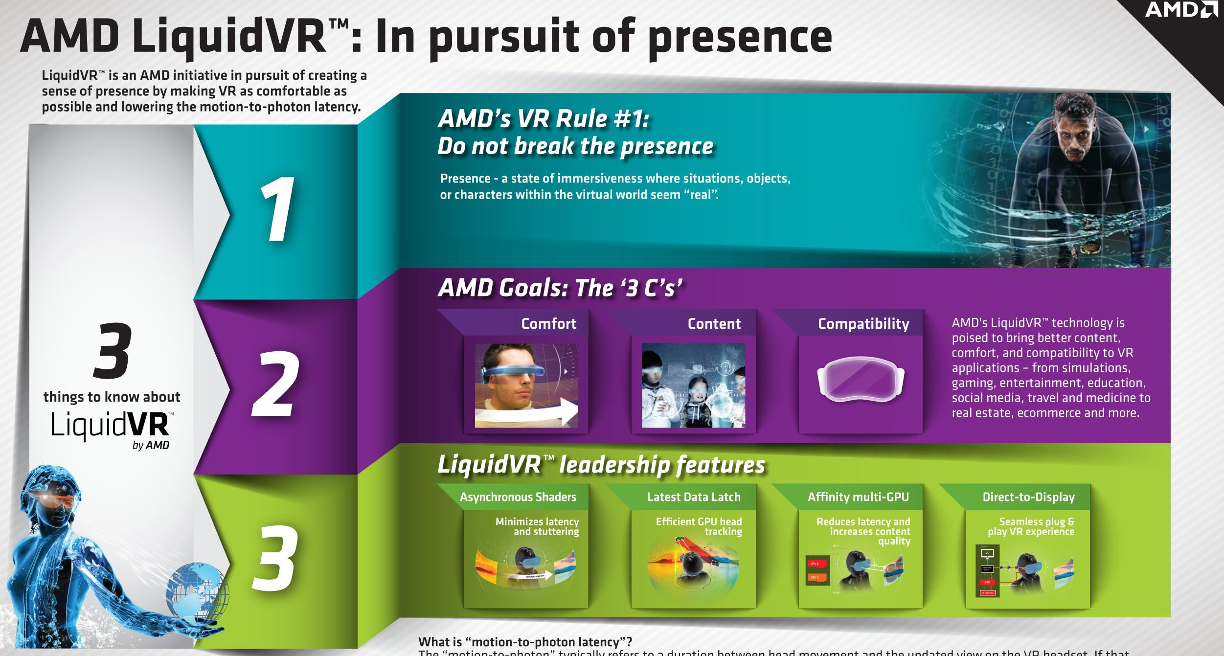
The "motion-to-photon" typically refers to a duration between head movement and the updated view on the VR headset. If that time is too long, motion-to-photon latency can disrupt good VR presence and may cause motion sickness and nausea.
